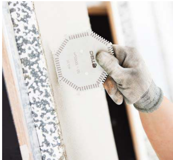
Layer-thickness measurement on reinforcing in the DAW Facade Technical Centre.
