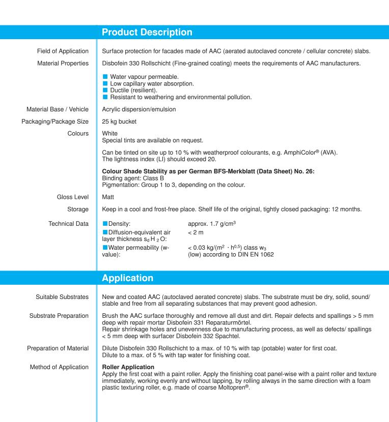
Fine-grained, acrylic emulsion-based coating for AAC (aerated autoclaved concrete / cellular concrete) slabs.
